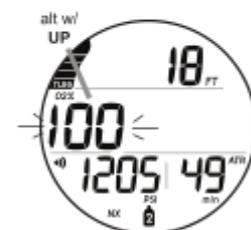
Fig. 116 - O2 ALARM MAIN (during Deco)
