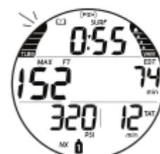
Fig. 43B - LOG DATA 1 (Deco, Nitrox)
