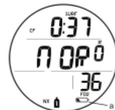
Fig. 2 - SURF MAIN (low battery warning)
