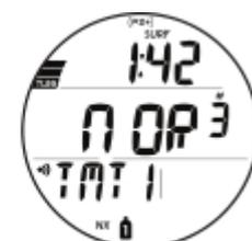
Fig. 6 - SURF MAIN (TMT low battery alarm)
