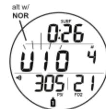
Fig. 110 - VGM MAIN (on surface > 10 min)
