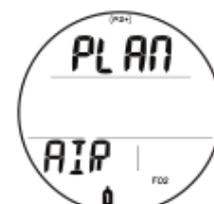
Fig. 39A - PLAN LEAD-IN (FO2 Gas 1 set for Air)
