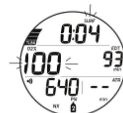
Fig. 117 - O2 ALARM MAIN (on surface, No Deco)
