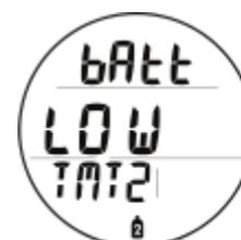
Fig. 5 - TMT BATT STATUS (low battery warning)
