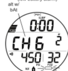
Fig. 4 - SURF MAIN (low battery alarm during dive)
