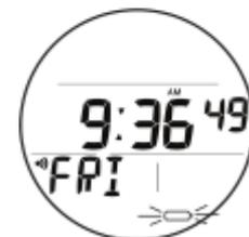
Fig. 3 - WATCH MAIN (low battery alarm)
