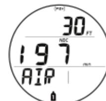
Fig. 40A - PDPS (FO2 Gas 1 set for Air)
