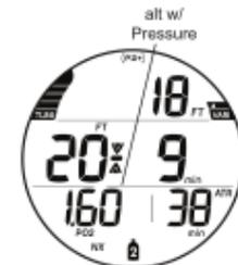
Fig. 113 - PO2 ALARM (while in Deco)
